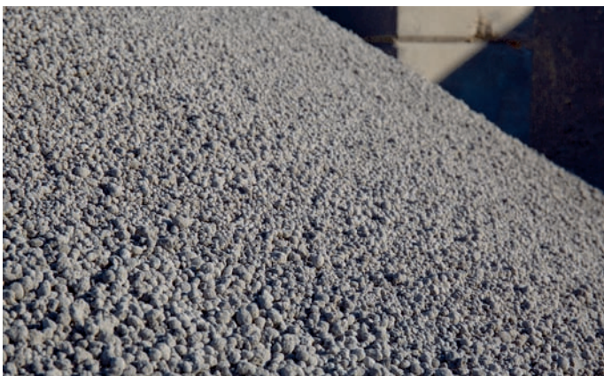
Carbon negative M-LS aggregate from O.C.O Technology is in demand as a sustainable building material
